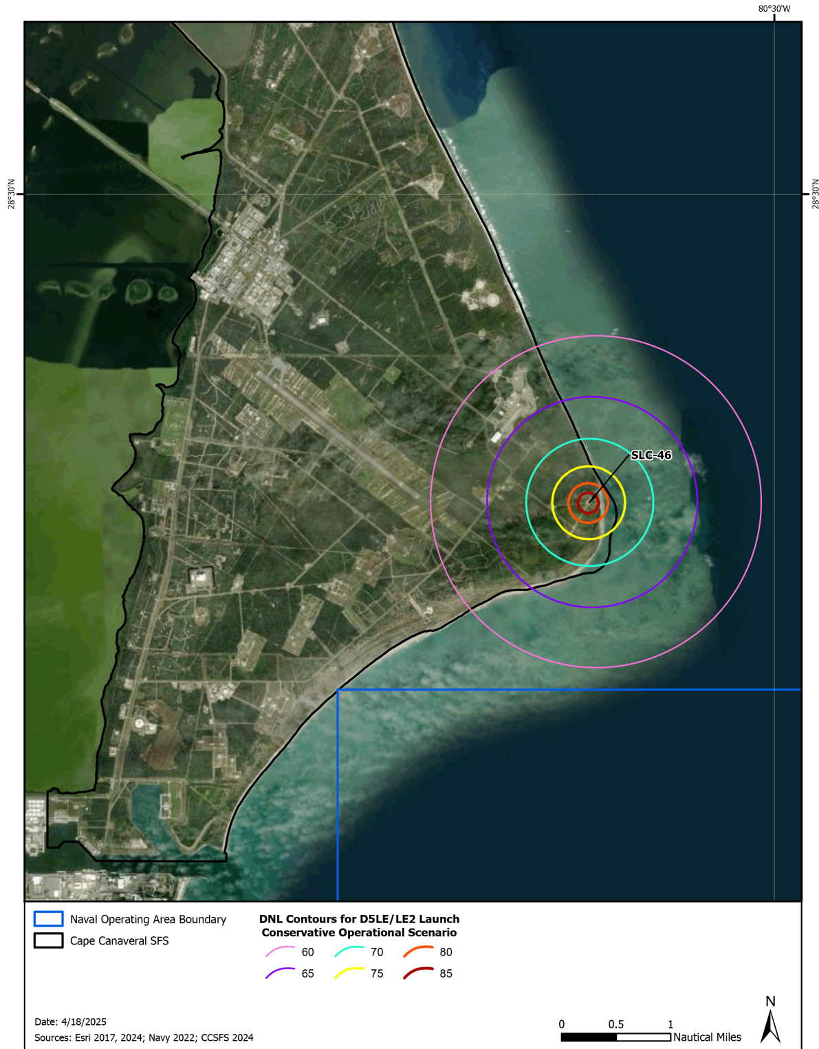
Figure E-3 DNL Contours for Proposed Weapon System Launch - Conservative Operational Scenario
